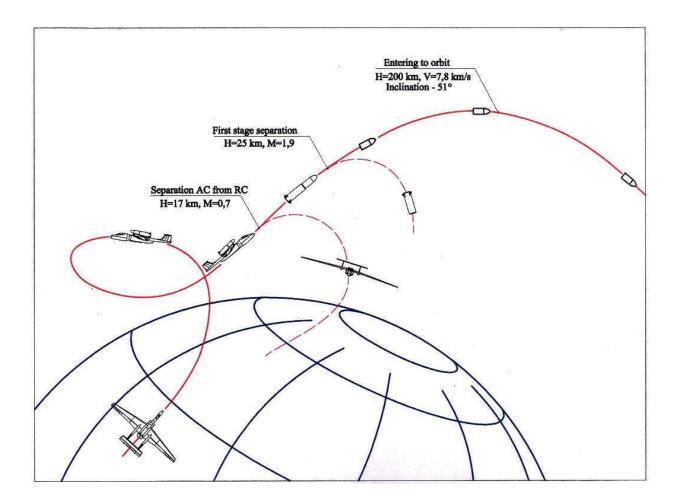
Calculations made for the rocket-carrier (RC) of 5500 kg mass, latitude of start  $47^{0}$  and inclination of orbit  $51^{0}$ , have shown that the mass of payload (micro-satellite plus acceleration block), which can be inserted onto 200 km circular orbit, ranges from 100 to 150 kg depending on the RC parameters.
